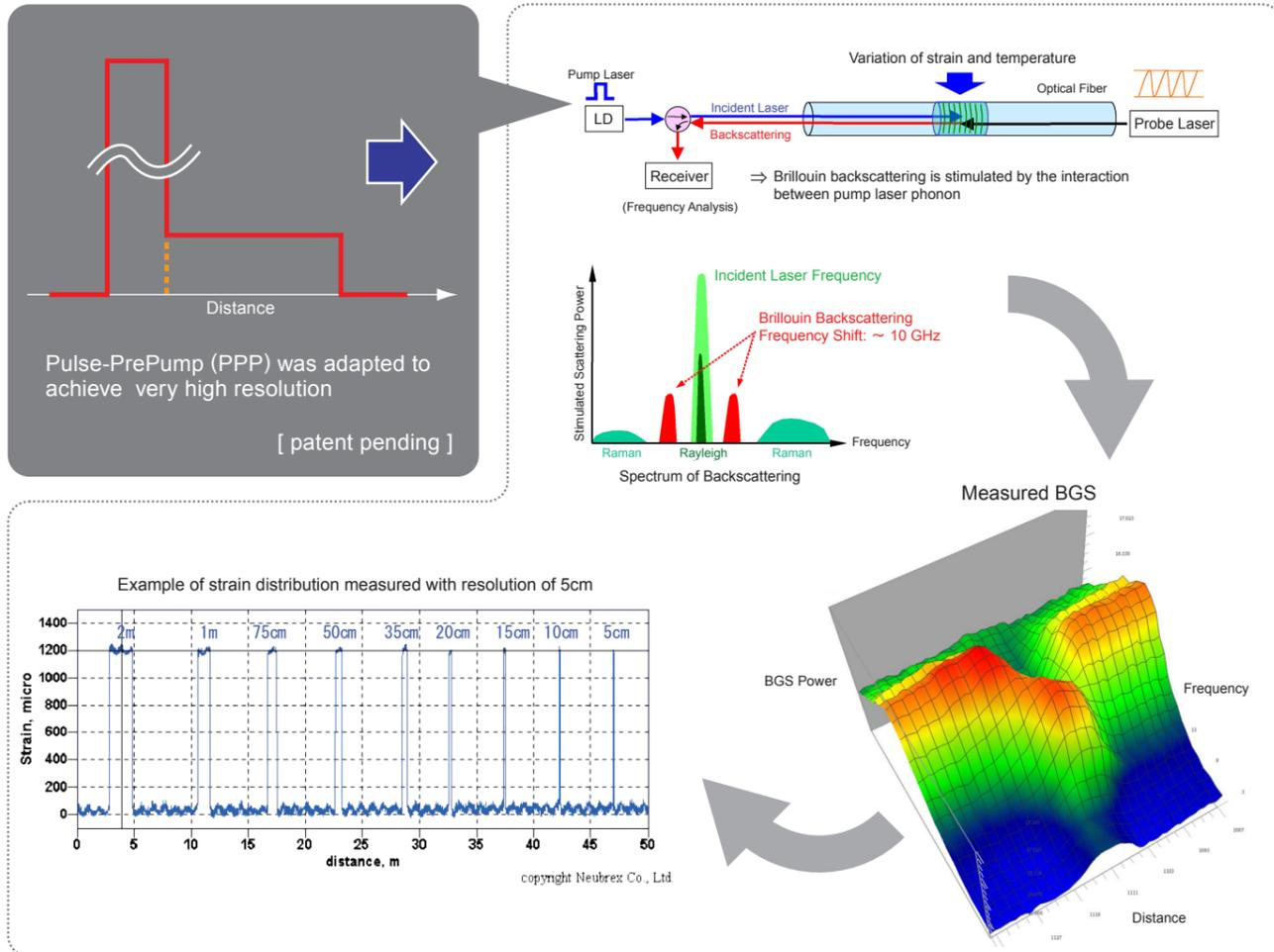
Neubrex technology of PPP-BOTDA successfully increases the spatial resolution and strain accuracy one-order higher than previous products. This is the only one technology in the world.
